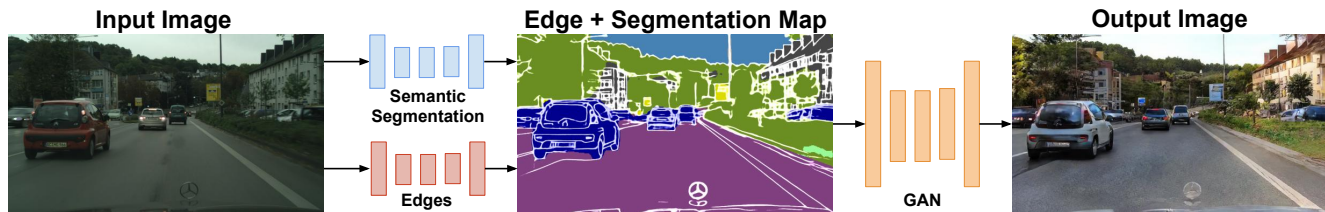
Figure 1: An input image is transformed into the output image using our framework: we first generate an EPS map as intermediate representation to then generate the output image in the target domain with an image-to-image translation GAN. Object classes of the EPS map are visualized based on the color scheme of Cordts et al. [10]. The input image shown here for illustration is taken from the Cityscapes data set.
