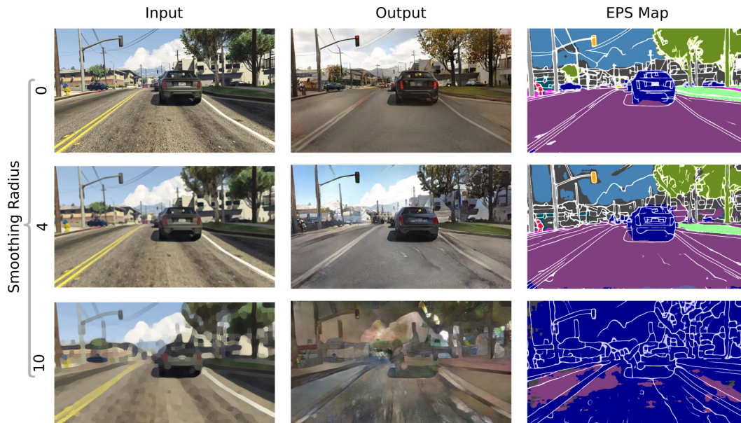
Figure 7: Illustration of the effect caused by smoothing the input image. A Kuwahara filter is applied with different radii. The input image is taken from the FCAV data set.
